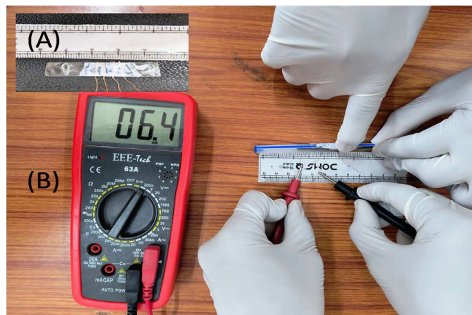
Fig. 7 (A) Prototype of piezoelectric sensor device. (B) Measurement on piezoelectric sensor device.
