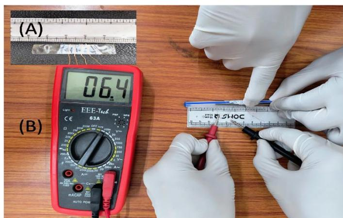
**Fig. 7** (A) Prototype of piezoelectric sensor device. (B) Measurement on piezoelectric sensor device.
