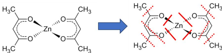
Fig. 9 Schematic diagram of breaking of zinc acetylacetonate.
