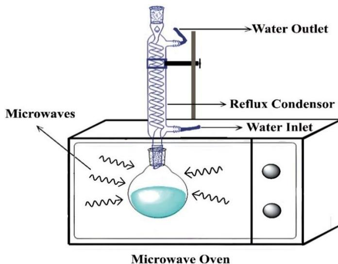
**Fig. 1** Schematic diagram of microwave synthesis method setup.
