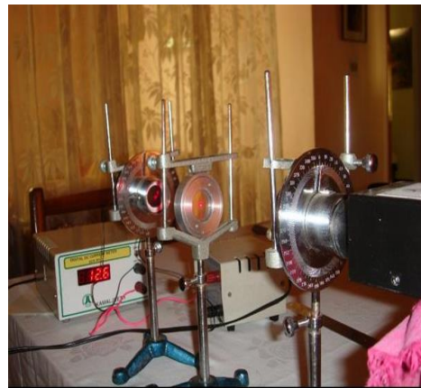
Fig 4: A QWP is inserted between the crossed polarizer and the analyser.
