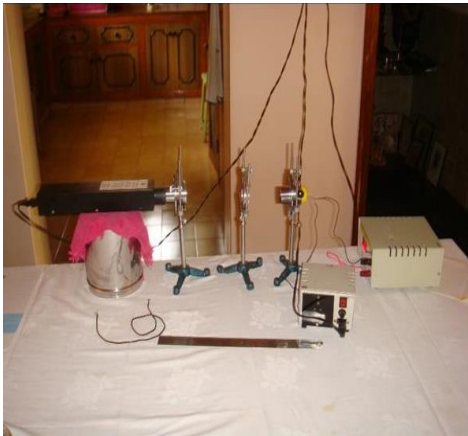
Fig 3: Laser, polariser, analyser and the LDR are placed coaxial at the same height. The LDR is connected to a DC supply and a milliammeter.
