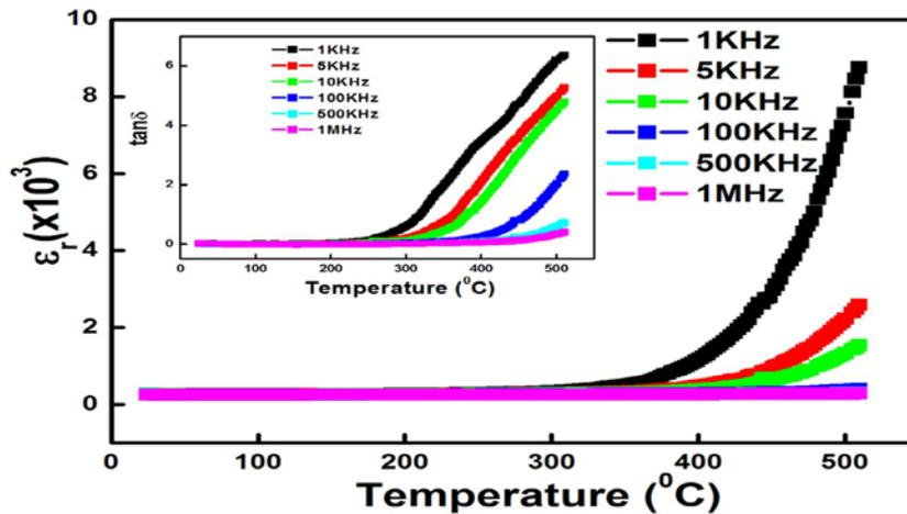
**Fig.3:** Temperature dependence of dielectric parameters
