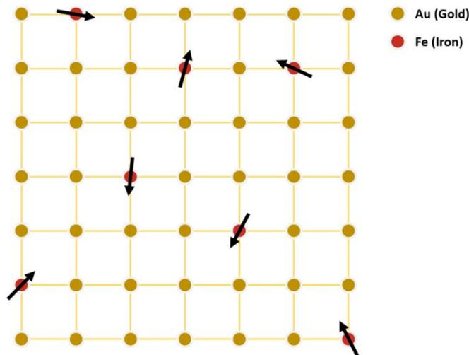
**Fig.2.** Schematic illustration of AuFe spin glass in which the iron atoms as magnetic impurities are mixed randomly to the nonmagnetic gold matrix. The spins associated with iron atoms represented by arrows are trapped in random directions.
