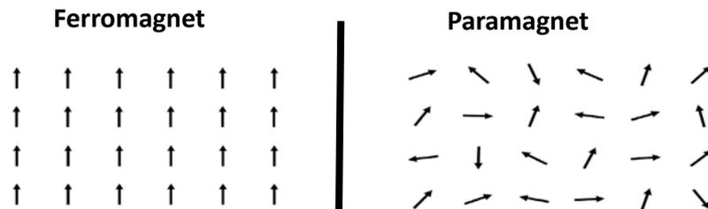
**Fig.1.** Schematic illustration of spin arrangement for a ferromagnet (spin-order phase) and a paramagnet (spin-disorder phase). The arrows indicate the spin magnetic moment at each atomic site.
