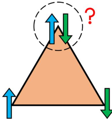
**Fig.3** depicts frustration in an antiferromagnetic triangular lattice i.e. when one spin points upward and the other downward, the third spin remains in a state of confusion as it cannot satisfy both of them simultaneously since adjacent spins prefer to point in opposite directions because of antiferromagnetic constraint.
