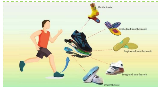
Figure 5: Diverse Applications of TENG for mechanical-to electrical energy conversion (enabled smart shoes).
