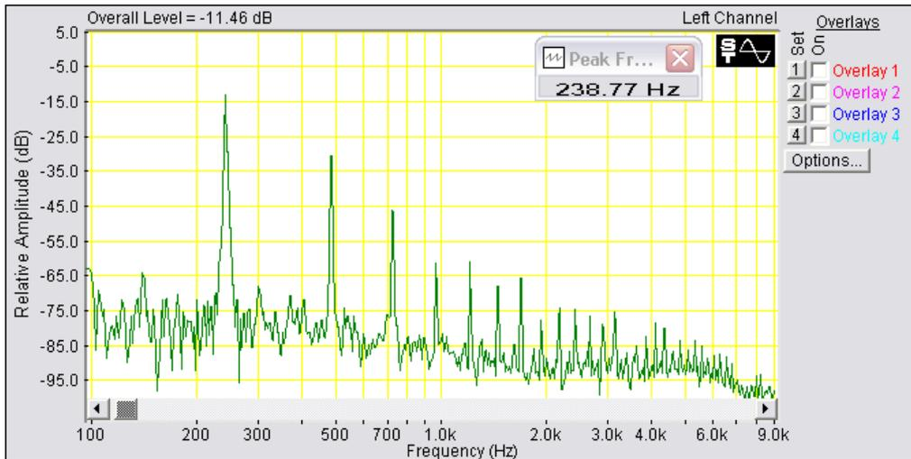
**Fig. 1(a).** Spectrum view of lip driven pipe of length of 110cm. & diameter 1.9cm.
