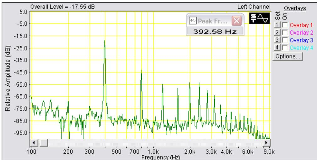
**Fig. 1(b).** Spectrum view at higher pressure with shifted frequency at the same tube length of 110 cm.
