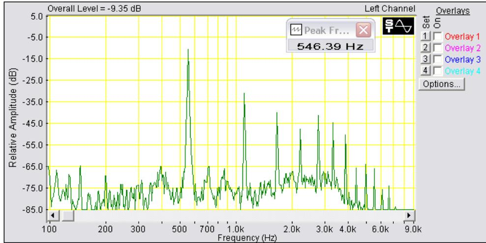
**Fig. 1(c).** Spectrum view at more higher pressure with shifted frequency at the same tube length of 110 cm.
